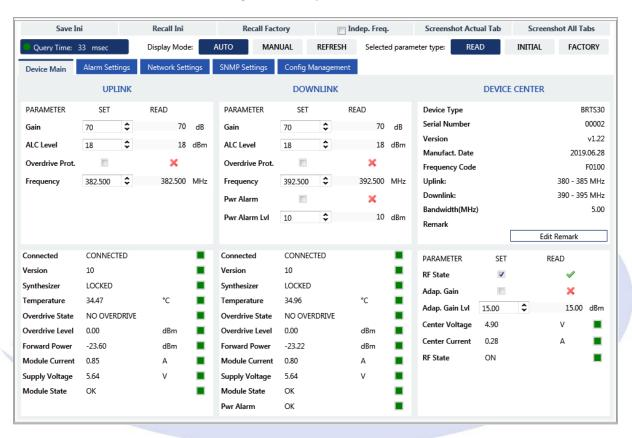
Some device parameters can only be monitored, while others can also be changed. There are two kinds of settable parameters: those that are saved immediately and those that are only saved when a specific 'save' command is issued to the device.
