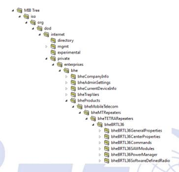
BHE MIB files have two parts: a part common to every BHE MIB file that contains common settings as well as general information about the company and the current device, and a device-specific second part. Note that the nodes and OIDs in the common part may change without notice — new parameters may be added or unused parameters may become deprecated.
