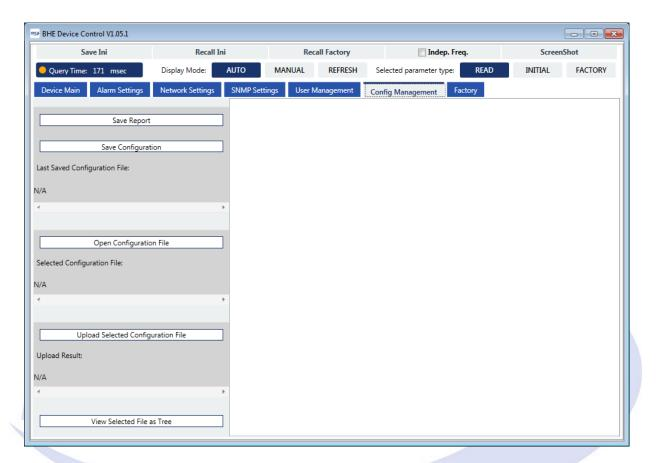
The Config Management tab in the control software allows managing the configuration of a single device. Configuration files are saved in human-readable XML format.
