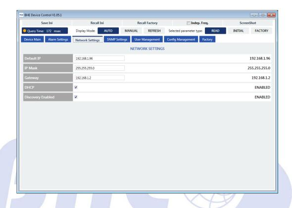
In the Network Settings tab, the user can set the network parameters of the device such as IP Address, IP Mask, Gateway address and DHCP operation. For a description of how these parameters determine the device's IP address, see chapter <a href="Ethernet Interface">Ethernet Interface</a>.
