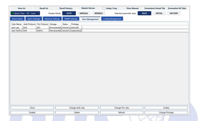
The User Management tab provides an interface for managing SNMP v3 users in the device. For an indepth description of user management, see chapter User Management.
